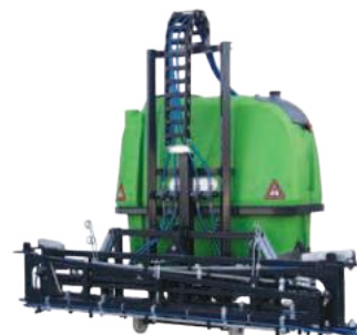
FOX RANGE : LIFTED WITH SELF LEVELLING MANUAL BOOM
