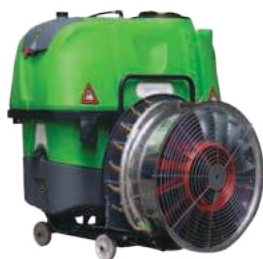
AXIAL ROUND FAN RANGE: V-BELT TRANSMISSION
